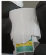
10. Adjust the PEEP according to local protocol
